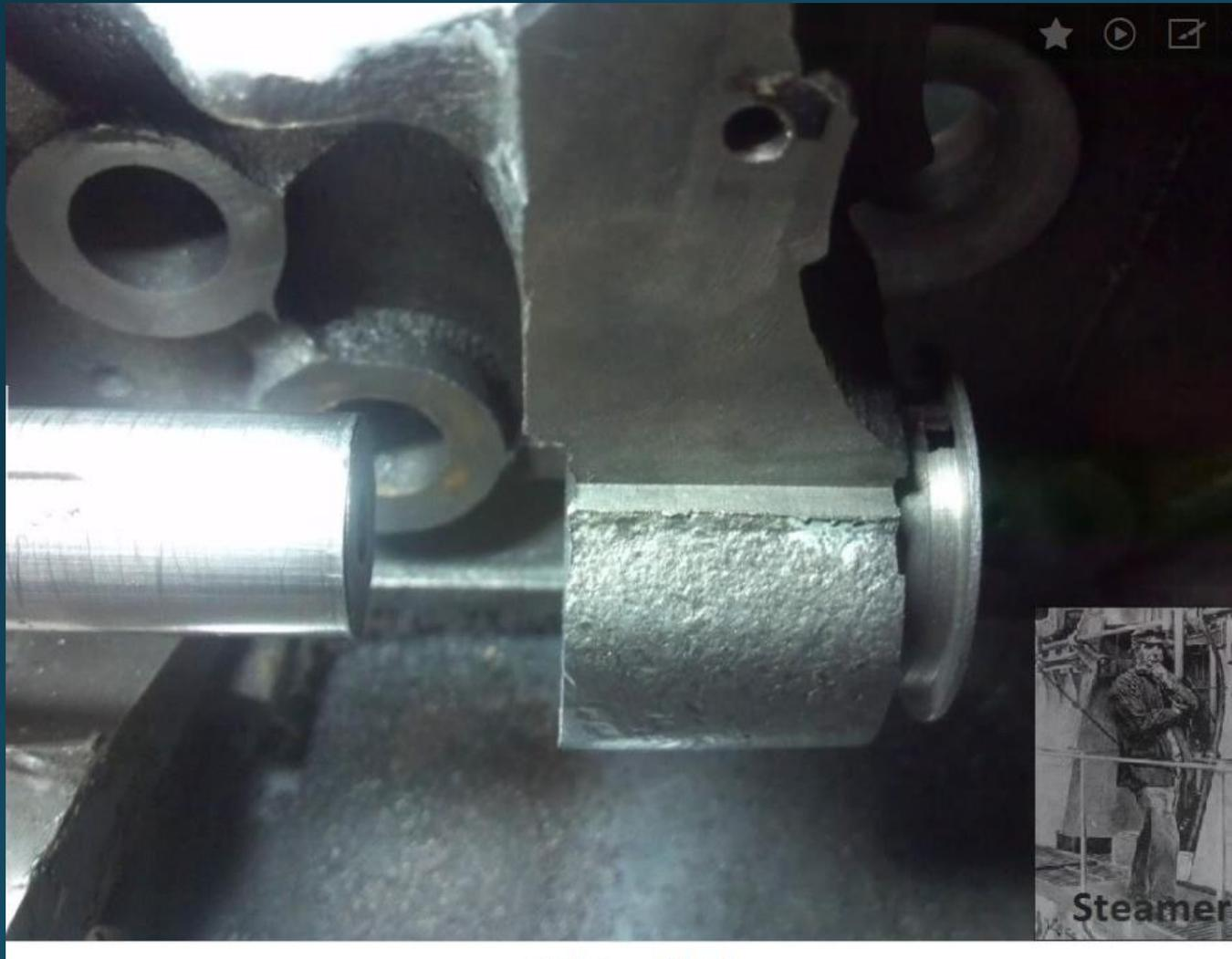
Bushing going into place prior to boring
