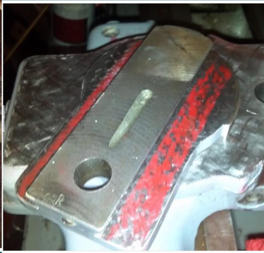
The flat ways of the compound showed to be still flat and in good condition. The top of the compound was not parallel to the base, so I scraped it in to within 0.0005". The ways on the compound base mated well with the Compound. Little work was needed
