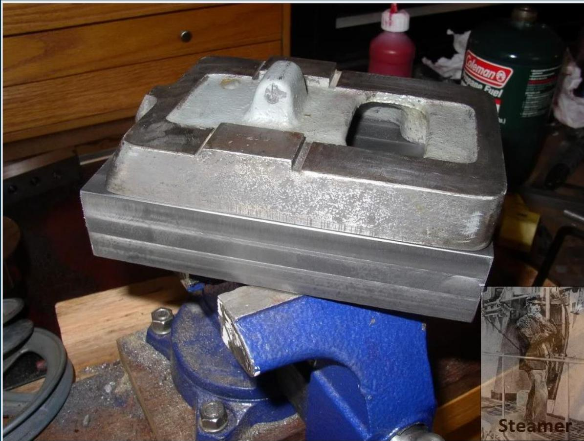
Existing one was 0.018" low and Worn with a severe "rocker".
