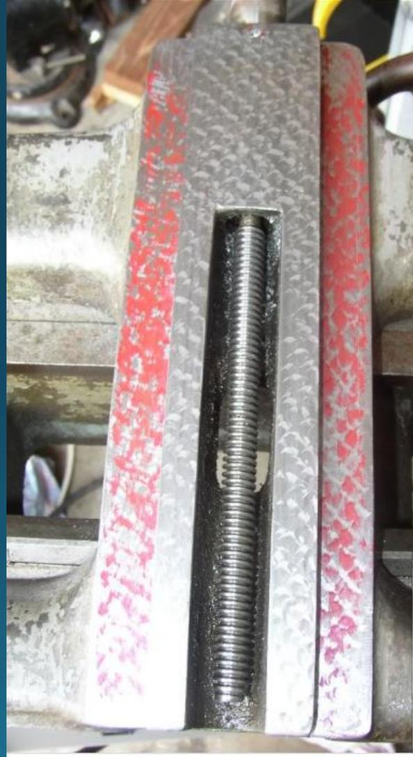
The saddle dovetail was a complete mess Very worn with ridges This photo was After several passes. Using the T slotted Cross slide as a gage for both surfaces Of the dovetails. There is enough float in The leadscrew nut in the vertical direction To accommodate quite a bit of adjustment.
