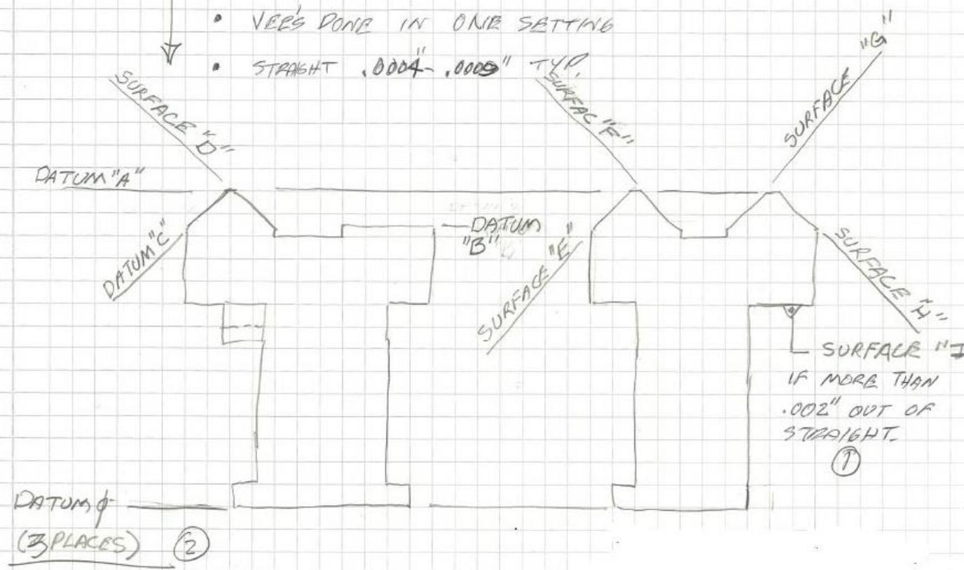
The key surfaces to be ground on the bed as conveyed to the grinding house.
