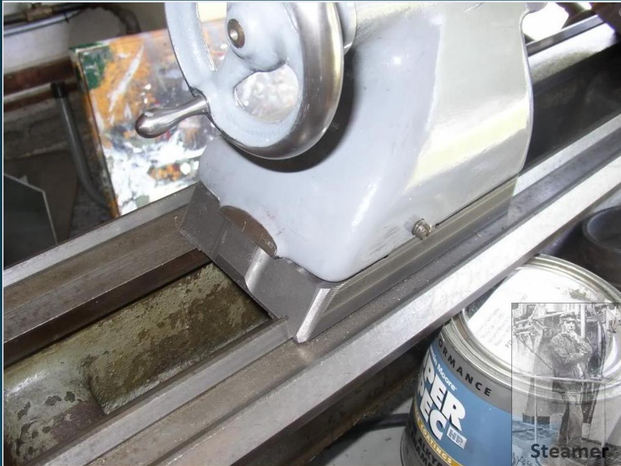
The base/top assembly machined to be 0.005" high. From there it was scraped into alignment in the Horizontal and vertical plane....but not yet.....8-)
