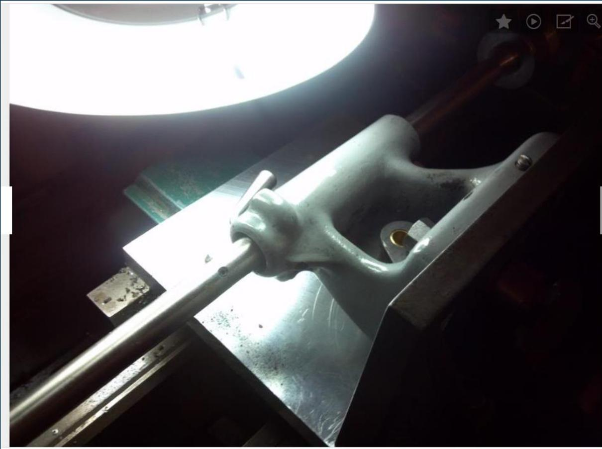
Set up a knee on the boring table. I bored the housing till it just cleaned up and no more being careful to align the base with the horizontal axis of the lathe.
